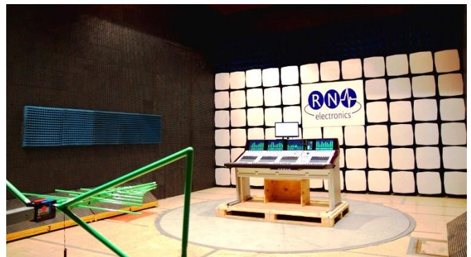
Testing at RN Electronics to EN 55032 of a Studer Vista X Broadcast Audio Console
